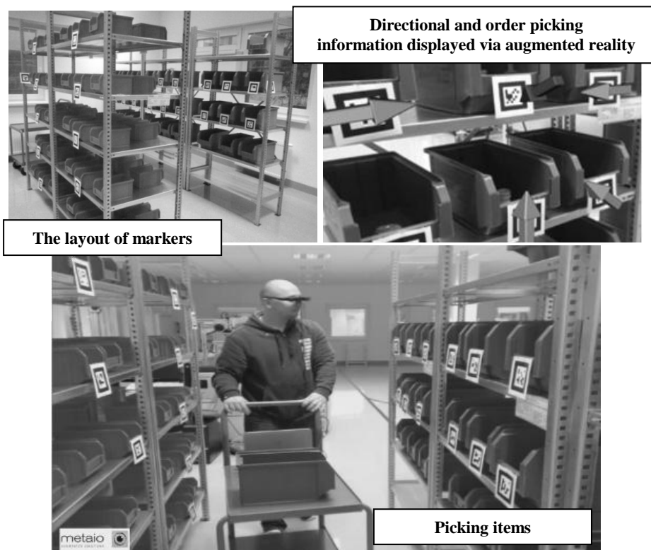
Fig. 6. Picking items with augmented reality (Mirandová & Gabaj, 2011)
