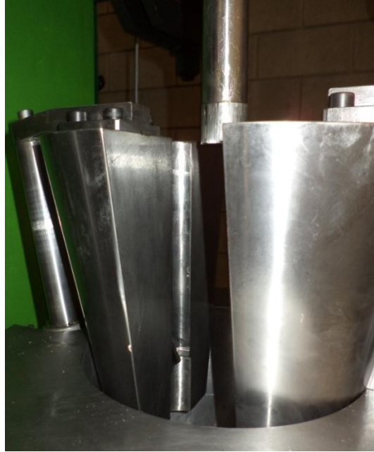
Fig. 11. Apparatus for split-die extrusion of twist drills
