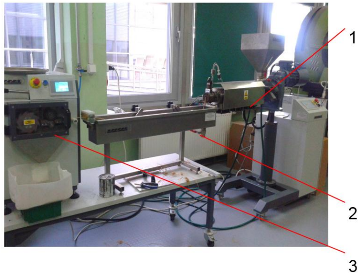
Fig. 2. Manufacturing of WPC composites: 1 – Zamak EPH-25 extruder, 2 – cooling bath, 3 – granulator
