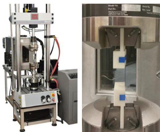
Fig. 1. a) MTS Bionix material testing machine, b) the tensile strength test gripping system
