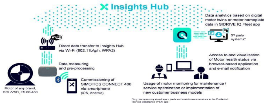
Fig. 2. IoT smart sensor architecture (Siemens Insights Hub)
