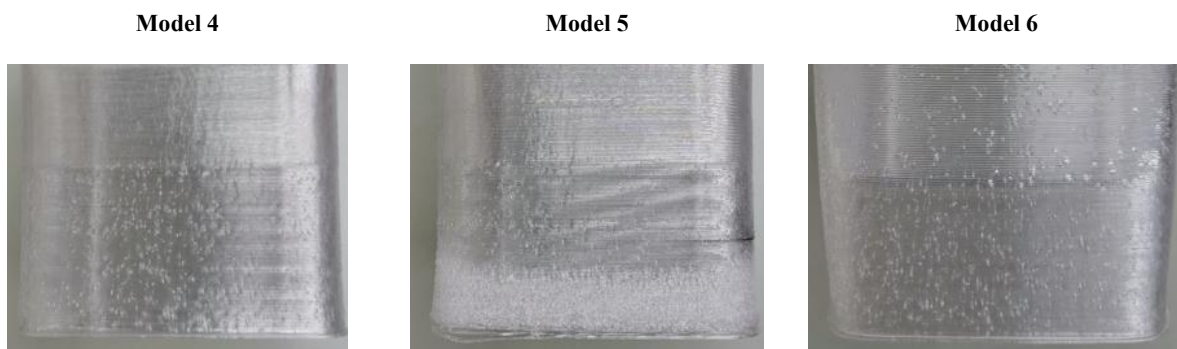
Fig. 7. Models obtained – variable values of the robot tool angles
