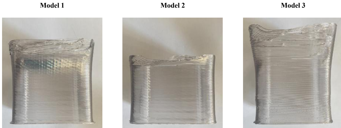
Fig. 5. Models obtained – constant value of the robot tool angles
