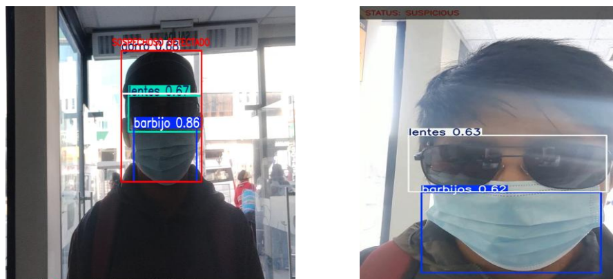
Fig. 9. Visualization of the ‘SUSPECT’ state generated by the YOLOv8-based analysis system
