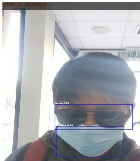
Fig. 13. Visualization of the 'SUSPECT' state generated by the Faster R-CNN-based analysis system
