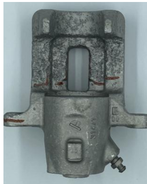
b) Severe body corrosion
