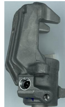
c) Damaged power-supply thread
