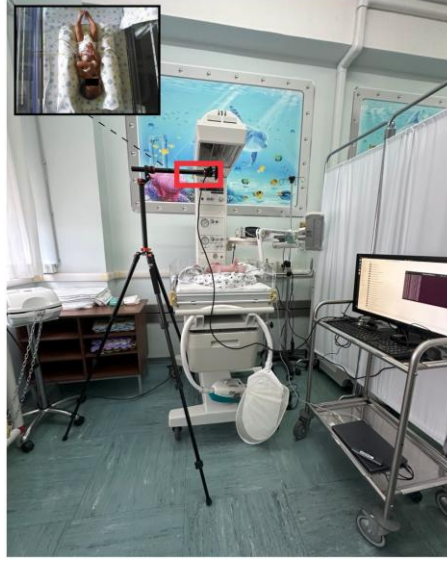
Fig. 2. RGB-D video acquisition setup. The RGB-D camera is positioned at about 50 cm above the infant’s crib and does not hinder health operator movements
