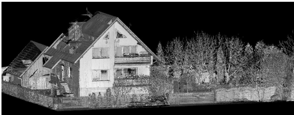
Fig. 1. Point cloud of a single-family residential building, source: own study
