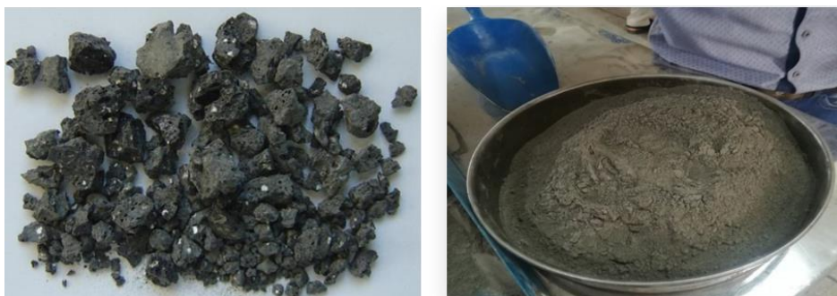
Fig. 1. a) Hospital waste ash obtained from NCPC, b) HWA after grinding in Los Angeles Abrasion Machine
