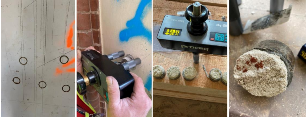
Fig. 3. Examples of photos from pull-off testing of plasters
