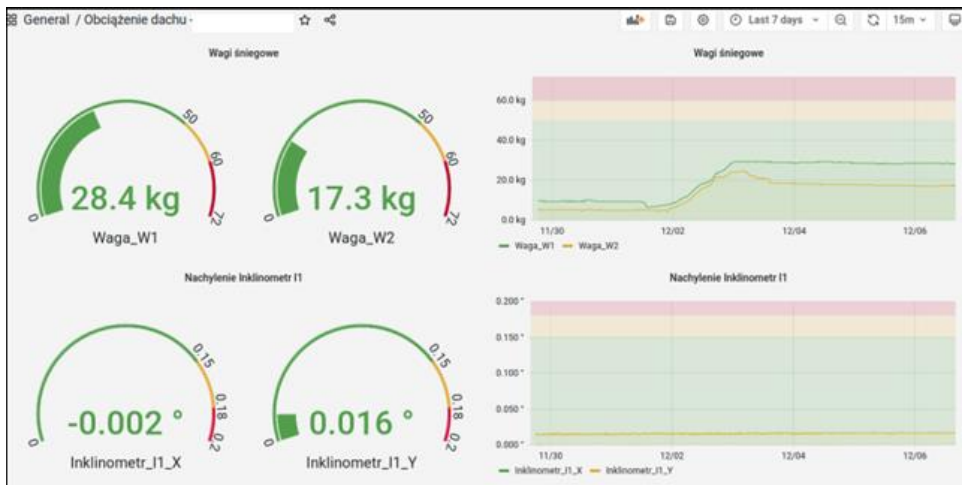
Fig. 14. Snow load information panel displaying two snow weights and roof structure element deflection for correlating result accuracy (own materials)
