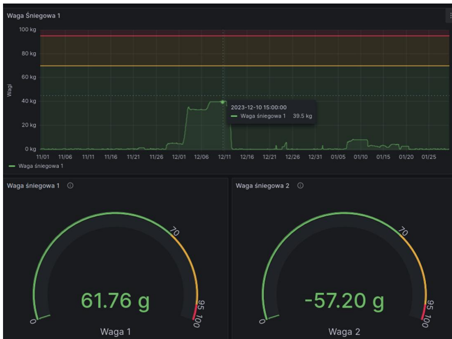
Fig. 11. Example of snow load observation history on the roof slope of a facility in Krakow (own materials)
