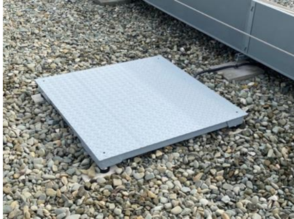
Fig. 5. Snow scale manufactured by KB-Projekty Konstrukcyjne Sp. z o.o. mounted on the roof (own materials)
