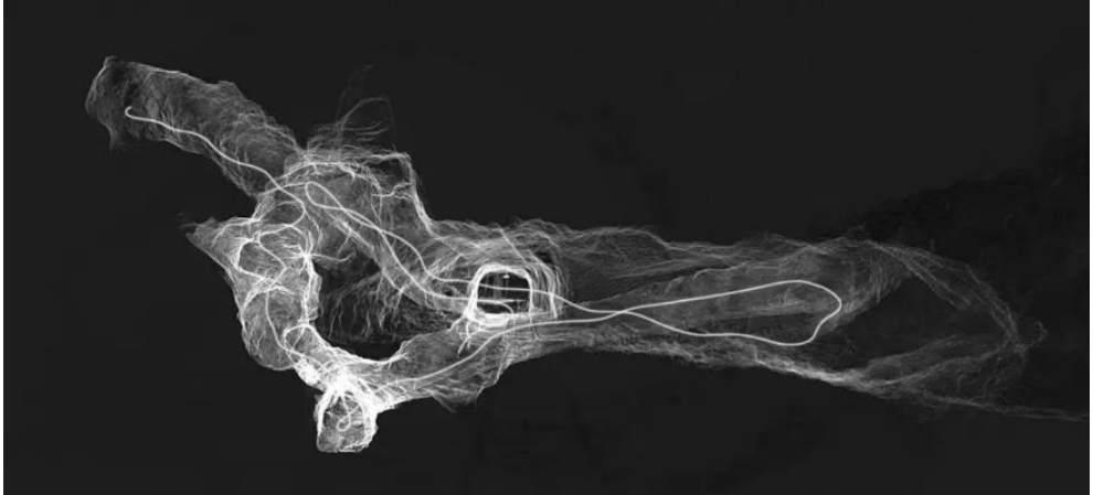
Fig. 10. Example of handheld laser scanning with a defined path [29]
