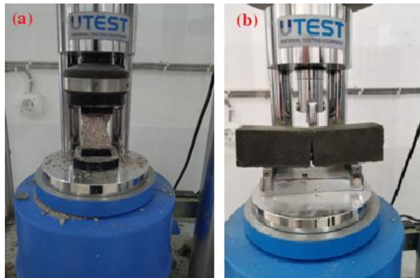
Fig. 4. Compressive and flexural strength tests of SCM. Source: own study
