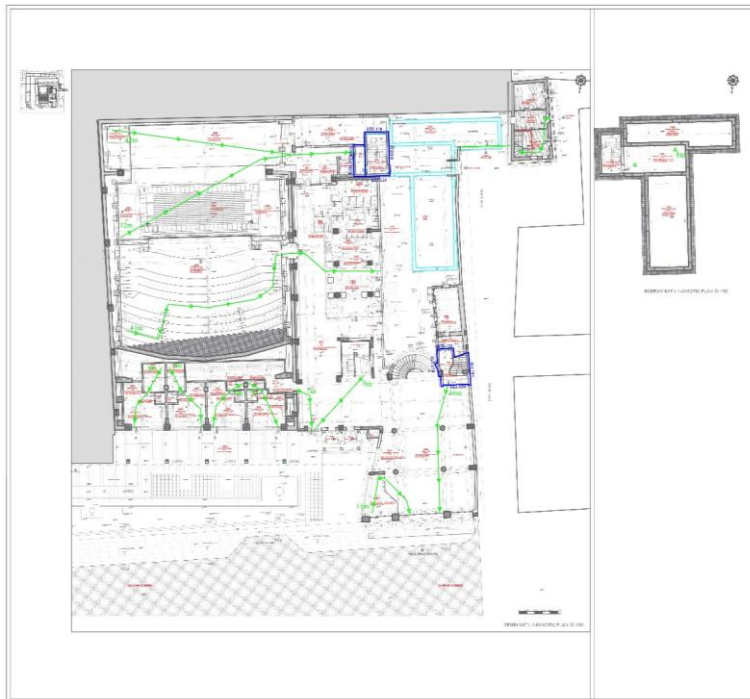
Fig. 4. Fire evacuation on the ground floor in the historic Yıldız Cinema (green lines indicate escape routes. The plan layouts on the right show the basement floor plans at -1.40 m). Source: The authors
