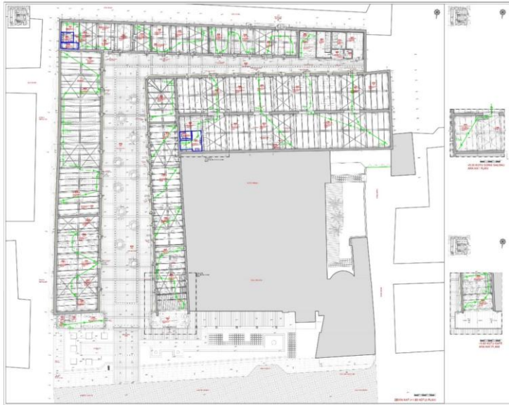
Fig. 3. Fire evacuation on the ground floor in the historic Bıçakçı Khan (green lines indicate escape routes. The plan layouts on the right show the mezzanine floor plans at +5.00 m). Source: The authors
