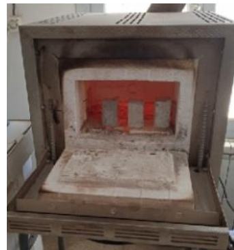
Fig. 6. Heating of specimens. Source: own study
