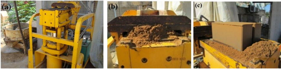
Fig. 3. Confection process of CSEB earth blocks. a-Machine of semi-automatic hydraulic press. b-rotate the dosing, c-block compact
