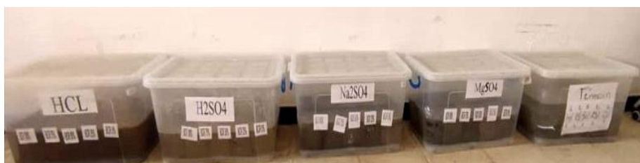
Fig. 8. Acid and sulfate attack test
