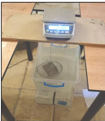
Fig. 7. Hydrostatic weighing of RCCP
