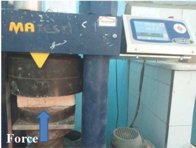
Fig. 5. Applying compressive force to clay bricks
