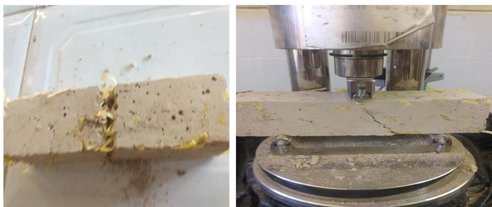
Fig. 12. Tensile strength test of adobe with LDPE plastic fibers
