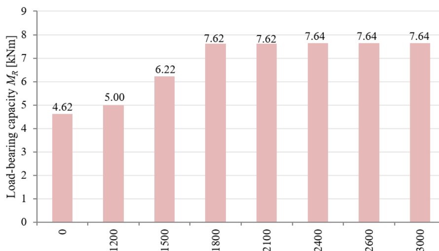
Fig. 10. Comparison of the load-bearing capacity of LVL beams reinforced with plates of varying length
