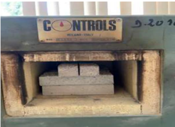
Fig. 6. Test of the effect of temperature on mortar mixes. Source: own study
