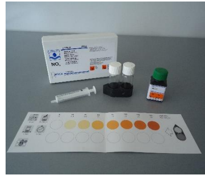
Fig. 8. Nitrate test Aquamerck® 111170. Source: own study
