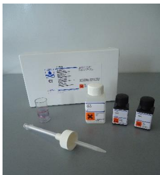
Fig. 7. Chloride test Aquamerck® 111106. Source: own study
