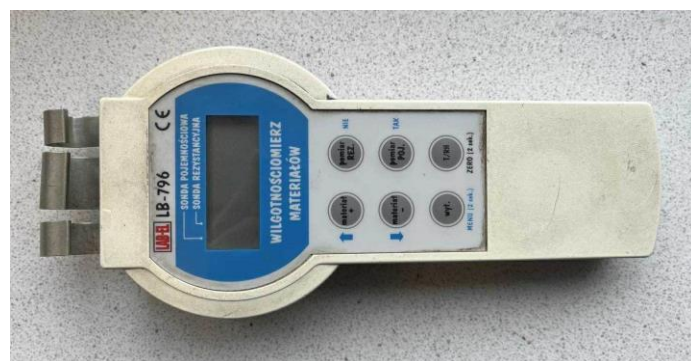
Fig. 6. Measuring device LAB-EL LB 796. Source: own study
