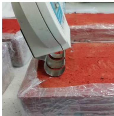
Fig. 5. Moisture measurement using the dielectric method. Source: own study
