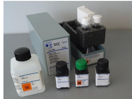
Fig. 9. Sulphate test Aquaquant® 14411. Source: own study
