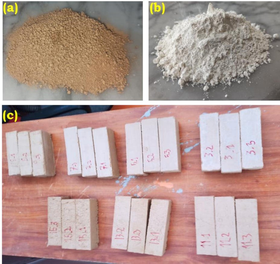
Fig. 4. Preparation procedure: a) soil, b) lime, c) specimens with dimensions of (4×4×16) cm 3
