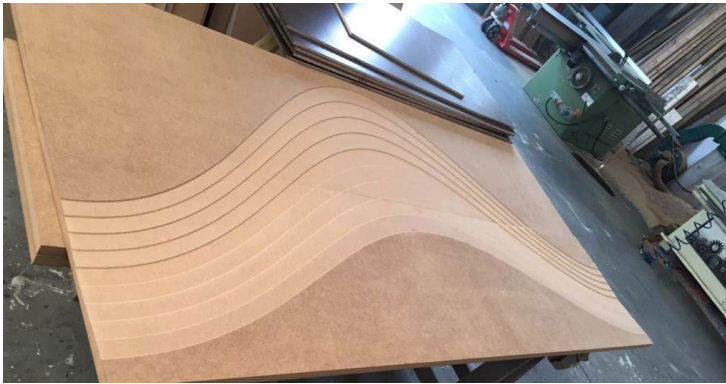
Fig. 7. The “WAVE” wooden positive just after the CNC milling process. Source: [Marcin Giedrowicz]
