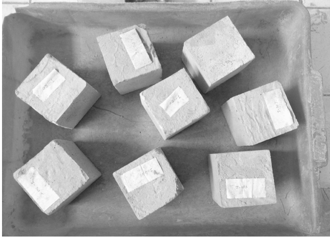
Fig. 7. Mortar cube specimens. Source: own study
