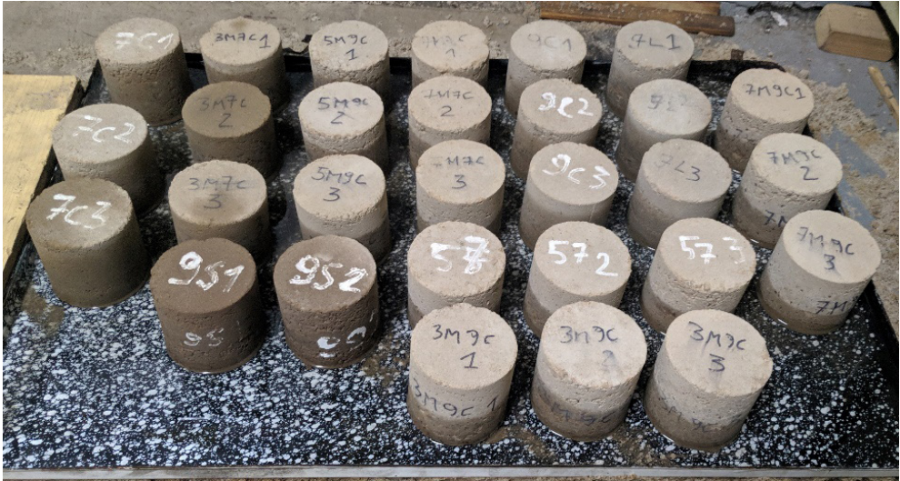
Fig. 6. Capillarity test – view 24 hours after immersion – Gp mixtures
