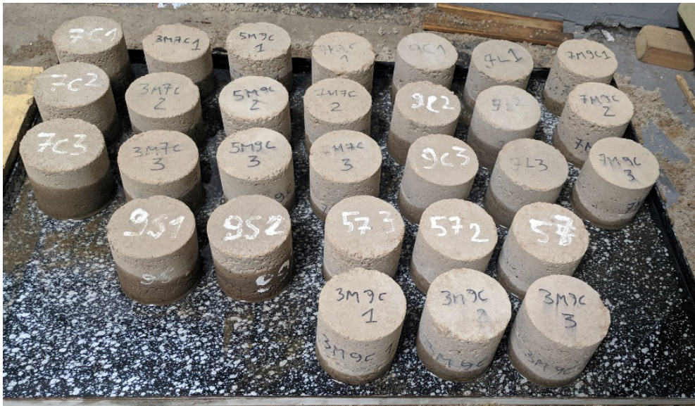
Fig. 5. Capillarity test – view after 3 hours from immersion – Gp mixtures
