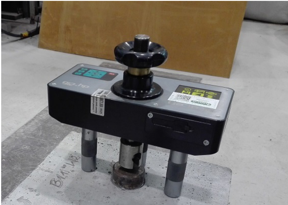
Fig. 2. A device used in the pull-off method (photograph by Dorota Michałowska-Maziejuk)
