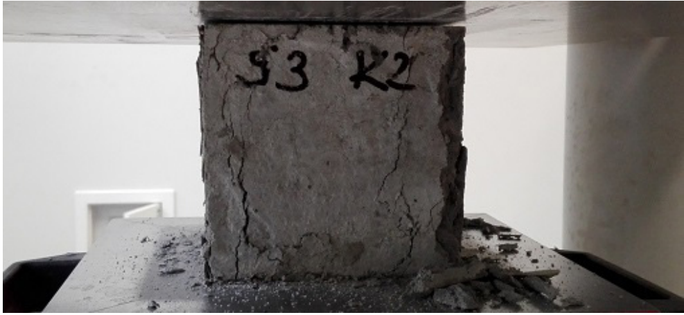
Fig. 3. Concrete specimen after compression test (photograph by Dorota Michałowska-Maziejuk)
