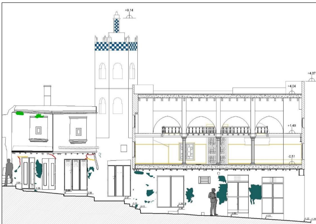
Fig. 7. Recorded deteriorations in the prayer hall and basement shops, source: the authors, 2018
