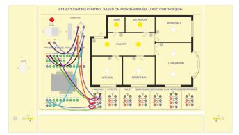
Fig. 9. Connecting patterns for ladder diagram at figure 8
