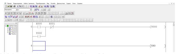
Fig. 6. The ladder diagram of program "Lighting control based on a programmable logic controller"
