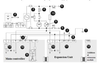
Fig. 4. Example of connecting a power supply to PLC: 1 - grounding: class 3; 2 - power supply; 3 - protective device; 4 - emergency stop; 5 - power indicator; 6 - load supply; 7 - built-in power supply; 8 - switch for the type of input switching; 9 - optocoupler; 10 - base block; 11 - extension block; 12 - extension module (ex. analog input); 13 - fuse (3 A)
