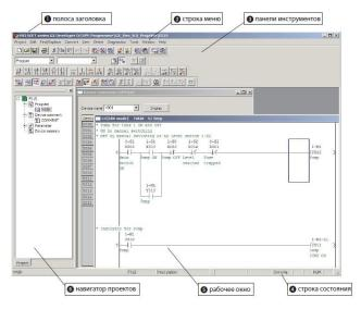
On this figure, for better visibility, the project is already open. After launching GX Developer, you only need to open an existing project or create a new project.
