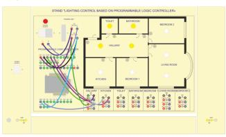
Fig. 7. Connecting patterns for ladder diagram at figure 6
