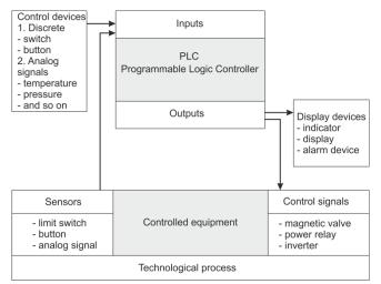
Fig. 1. Functional diagram CS on PLC base
