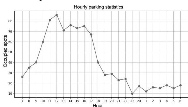
Fig. 2. The result of modeling the parking lot operation taking into account changes in traffic intensity during the day
