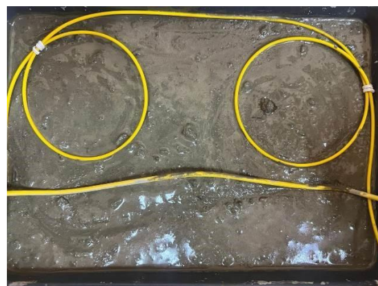
Fig. 2. Optical fiber integrated into concrete
