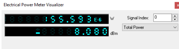
Fig. 10. Total electrical power for a soliton PAM modulation scheme with a 65 mA SOA injection current over a 200 km fibre length
