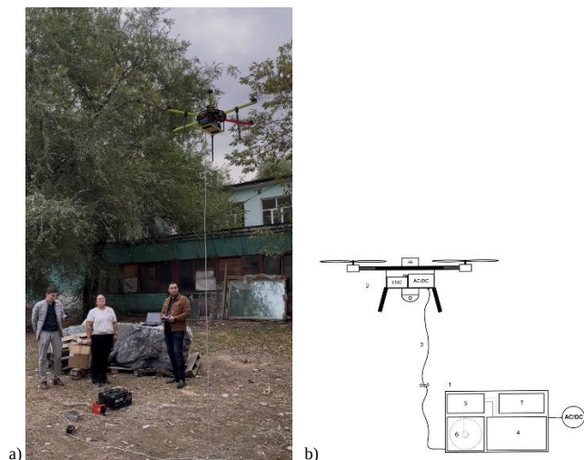
Fig. 5. Tethered UAV power supply system with a multilevel inverter and telemetry-based monitoring of power parameters: (a) experimental field testing of the tethered UAV platform, b) structural diagram of the proposed power supply system
