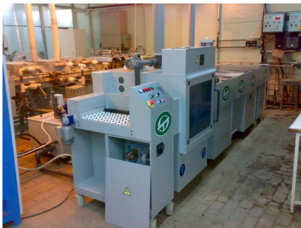
Fig. 13. A photo of the whole etching module (in the centre) and its loading module (in the front), rinsing and drying modules at an enterprise; the electrical control system is seen at the loading module (where circuit boards are loaded) with its buttons for turning on and off distinct components of the system, and signaling the system states and issues (for instance, the water consumption rate sustainability)
