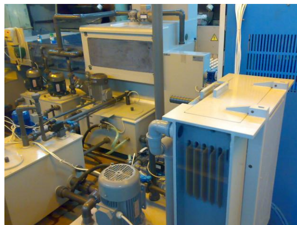
Fig. 14. A photo of the compact etching solution regenerator (on the right), where parts of the etching module are seen on the left, with a productivity of the printed circuit board (substrate) etching line of 14 m 2 /h
