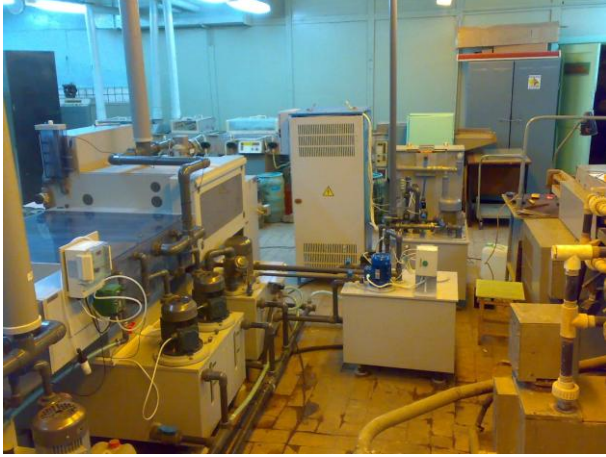
Fig. 9. A photo of industrial operation of the etching line with integrated electrochemical regeneration at an enterprise, where the power box used for the regeneration unit is seen; the three tanks with solutions are seen in the front along with the pumps mounted above the tanks
