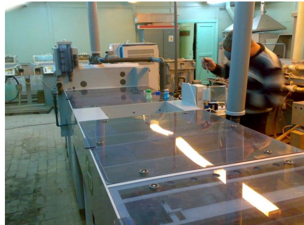
Fig. 11. A photo of the conveyor of circuit boards under acrylic glass, where the worker observes and adjusts the technological parameters of the etching line (the etching module is seen farther in the background)
