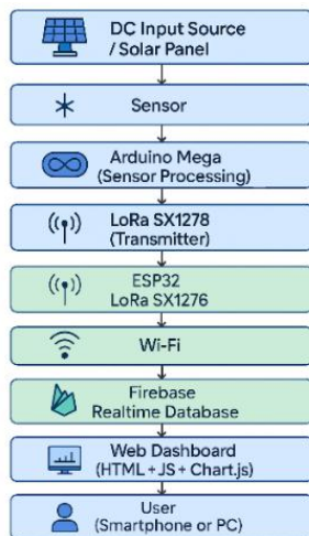
Fig. 1. Proposed system architecture integrating fuzzy logic diagnostics with LoRa-based monitoring
