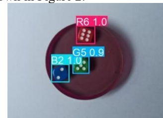
Figure 2: Example detection result obtained during testing of the YOLOv8 model. Bounding boxes indicate detected dice faces and their predicted class labels
