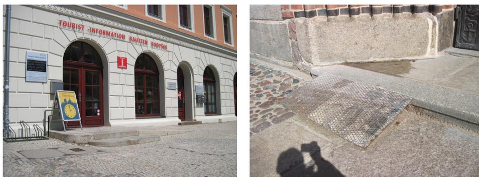
Fig. 3 A ramp incorporated into the surroundings of the historic building and a temporary ramp made of steel. (photo by the author)
