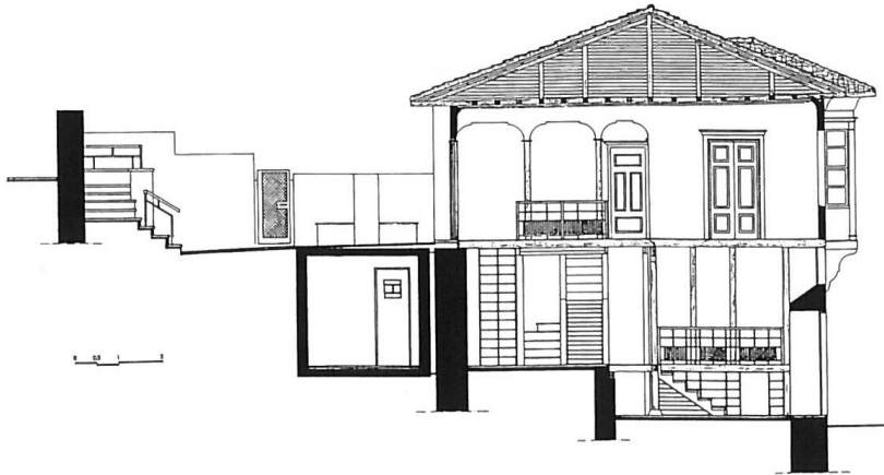
Fig. 3. House on 19, Epimenidou Street, cross-section, displaying the arrangement of the lavatories in a blind extension of the ground floor, dug into the ground rise. Source: Anagnostidis, M., Doussi, M., Chatzopoulou, O. et al. (2001), 183 (Fig. 62)
