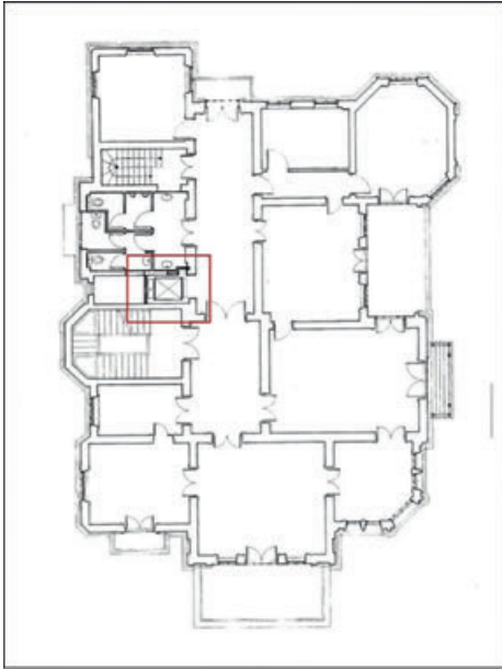
Fig. 22. The Former Ahmet and Giousouf Kapandji Mansion, plan of the first floor, with the location of the passenger lift.
