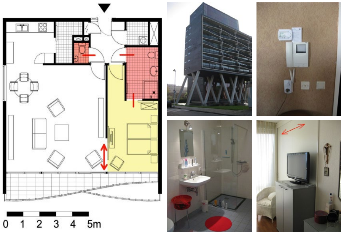
Fig. 2. An example of a flat with service – with one bedroom. The bedroom is connected, with the living room through mobile walls. Bathroom connected to the bedroom by additional sliding doors. De Plussenburgh, Rotterdam, the Netherlands. Graphic and photo – author.
