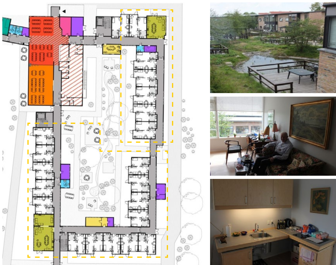
Fig. 3. Housing form with care – groups of flats with additional common spaces and staff points (marked with dotted line). The division is also reflected in the body of the building. Common areas include terraces. Rosenlund, Mørkhøjvej, Denmark. Graphic and photo – author.
