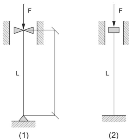
**Fig. 6.** Ways of fixing element ends, Source: own research
