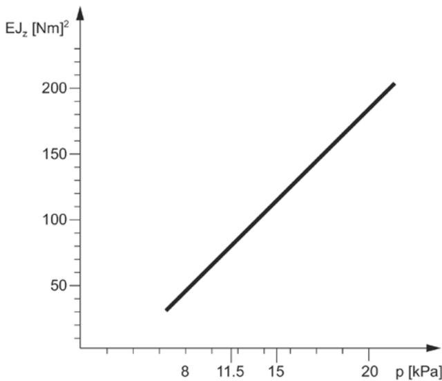
**Fig. 7.** Bending stiffness versus pneumatic element internal pressure. Source: own research.
