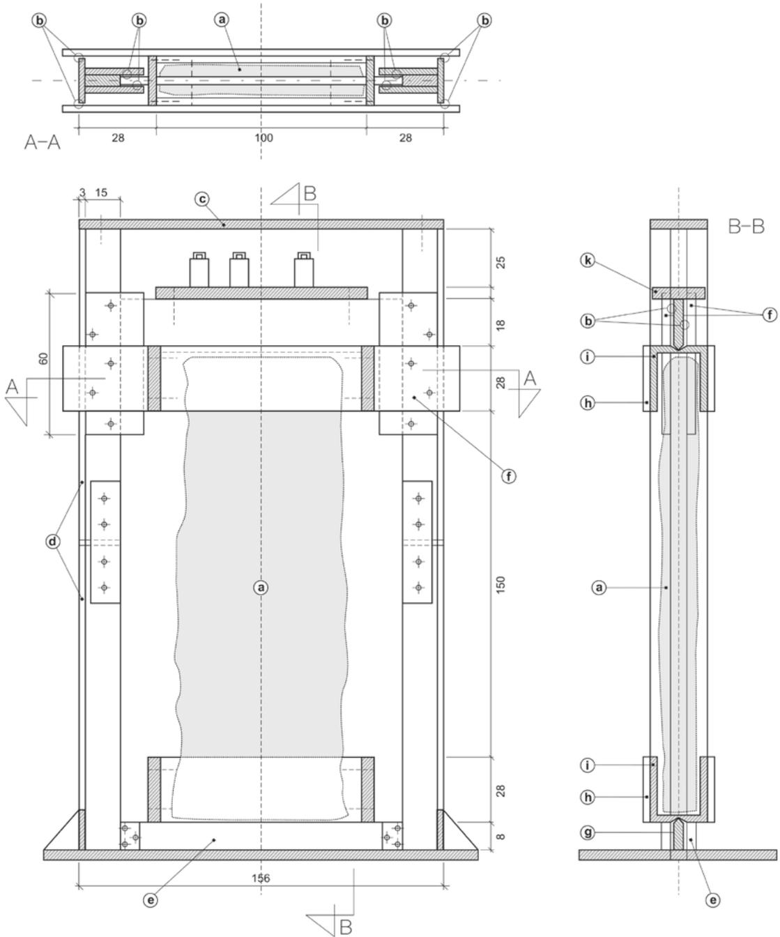
**Fig. 10.** Loading system (a – Inflatable mattress, b – Sliding gaps, c – Stiffener plank, d – Members joined together at mid height, e – Fixing element, f – Guides, g – Permanent element, h – Screwed-on plank, i – Box, k – Moving element). Source: own research.
