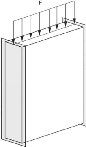
**Fig. 3.** Compression loading scheme for pneumatic component. Source: own research.
