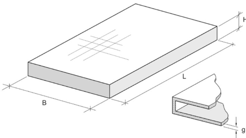
**Fig. 1.** Dimensions of pneumatic structural component and directions of plate anisotropy. Source: own research.
