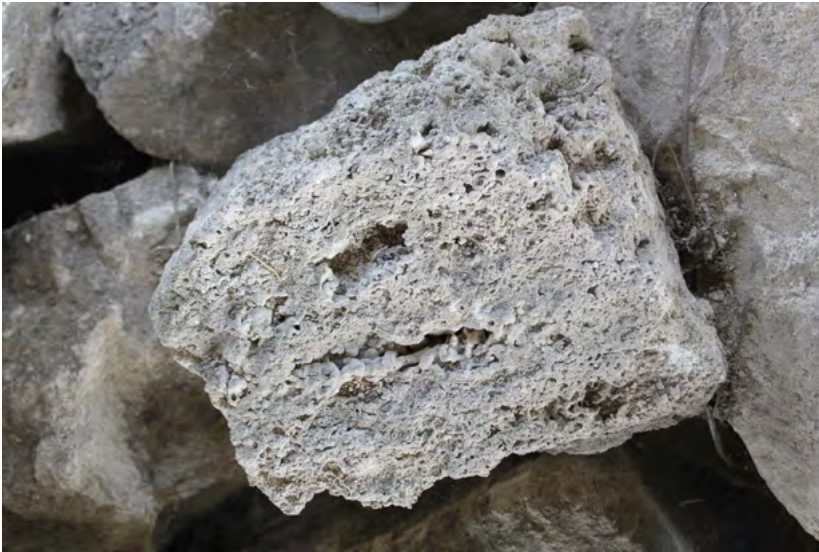
Fig. 11. Travertine block with a complex heterogeneous porous structure (village Krylos)
