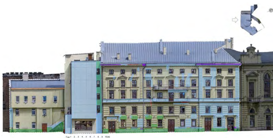
Figure 14. Graphical inventory of damage on the southern façade. Source: Authors
