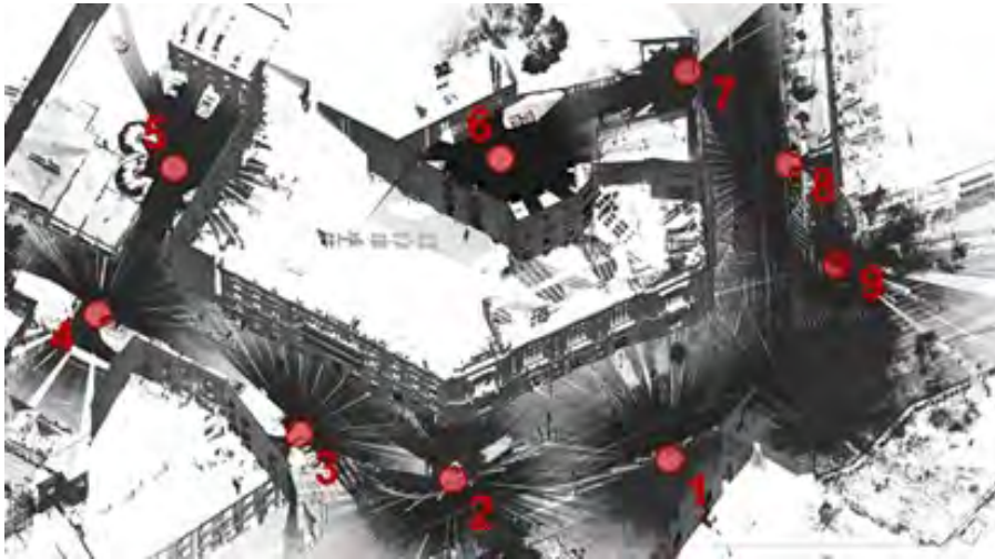
Figure 7. Layout of laser scanner stations. Source: Authors
