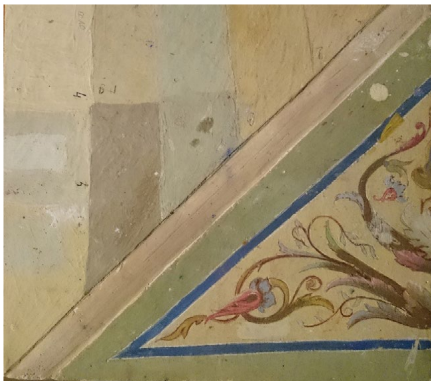
Fig. 11. Tests on colour and the property of casein and cretaceous-glime paints and their compatibility with each other and the basis (author – S. Hetmanchuk).
