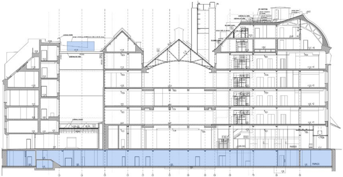
Fig. 9. Feniks Department Store refurbished in 1997–2015 – section drawing, plant rooms indicated with light blue color (by Kirschke Pracownia Projektowa).
