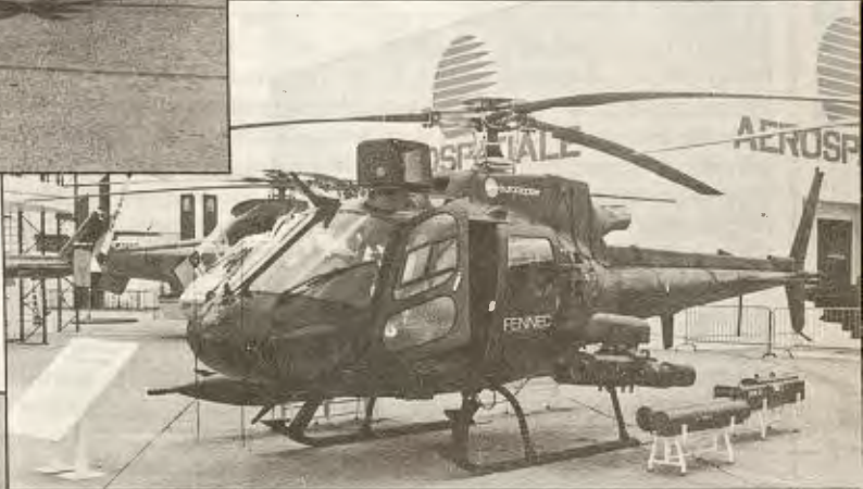
Bojowy Eurocopter Fennec (d. Aerospatiale AS 550/555), czyli nowe wcielenie znanego AS 350 Ecureuila
