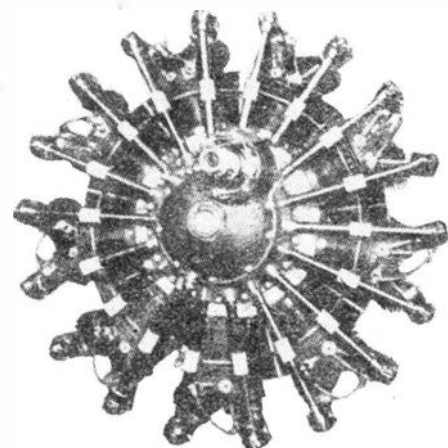
Rys. 3. Nowkuńskiego GR-760 280 KM do RWD-9. Nowkuński's GR-760 280 hp engine for RWD-9 aircraft
